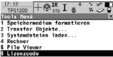
The screenshot shows the top status bar of the TPS1200 software with the time 17:12 and the device name TPS1200. Below it is the 'Tools Menü' window, which is a list of options: 1 Speichermedium formatieren, 2 Transfer Objekte..., 3 Systemdateien laden..., 4 Rechner, 5 File Viewer, and 6 Lizenzcode. The '6 Lizenzcode' option is highlighted with a black background and white text. |
