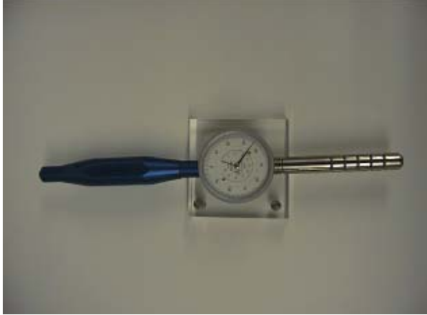
No. 1 Deflectometer (Messuhr) Huggenberger Zürich, Jointmeter JM 3D
