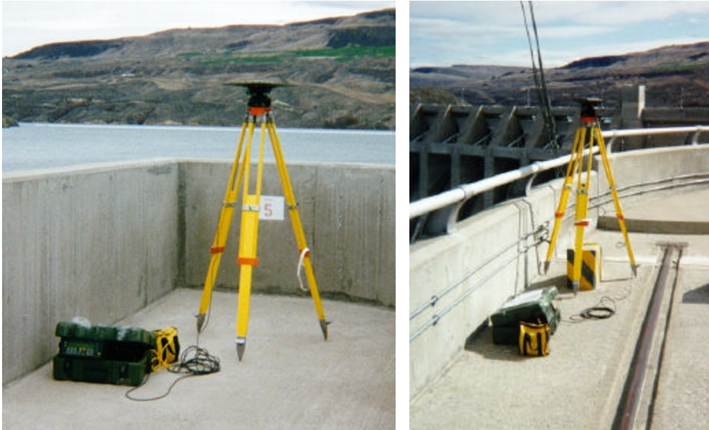
Figure 3-4. GPS equipment setup on a concrete hydropower dam - spillway and intake structure
