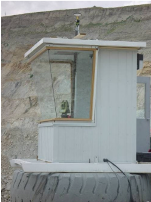
Figure 5 A shelter with RTS and GPS in the Valley Pit
