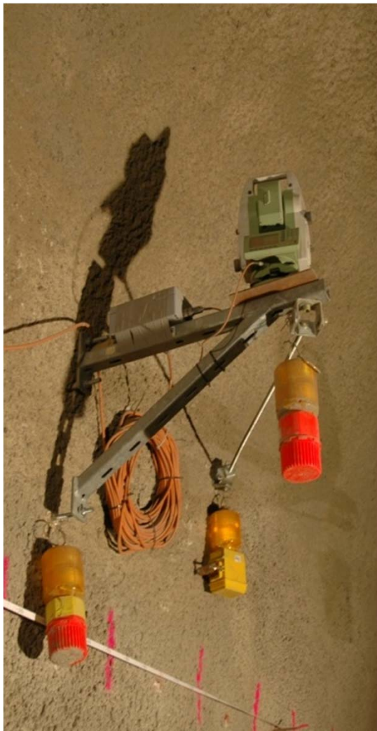
Console with total station, Mt. Terri Project. Source: Stephan Schütz
