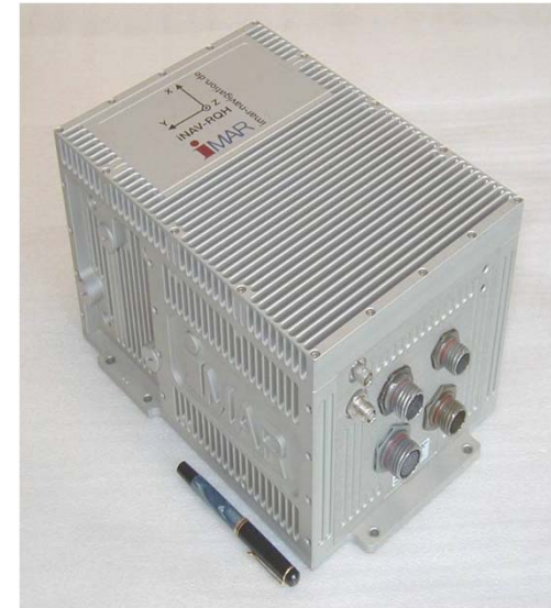
IMAR IMU with QA2000 and GG1320. Source: www.imar-navigation.de
