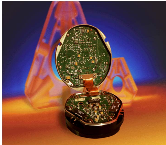
Honeywell GG1320 ring laser gyro. Source: www.honeywell.com
