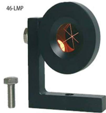
Typical mounting „L-supporter“ for monitoring.
